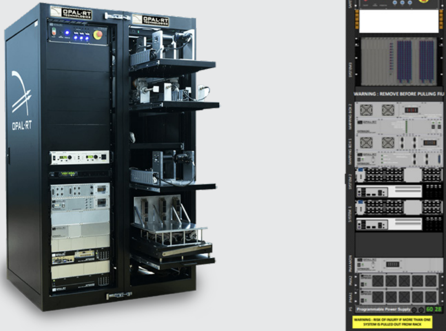
Figure 16 – OPAL-RT's test bench can be fully customized to test not only the FADEC but also any actuator, valves and sensors.
