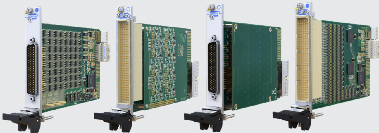
Figure 10 – Industrial digital I/O family for digital signal generation and sensing, for fault-protected testing applications.
