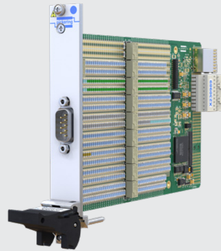
Figure 7 – Pickering Interface's PXI/PXIe 15 W Programmable Resistor Modules can be programmed in increments down to 0.125 \Omega with resistance values from 1 \Omega to 395 k \Omega depending on variants.
