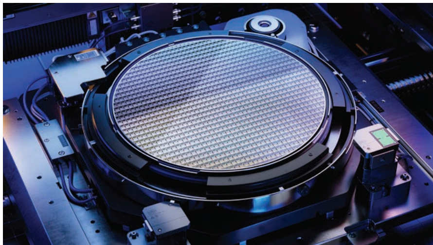
Figure 1 - A manufactured wafer prior to Wafer Acceptance Testing
