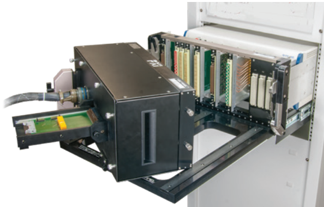
Fig. 7.6 - Mass Interconnect Connection for PCB Test (MAC Panel)
