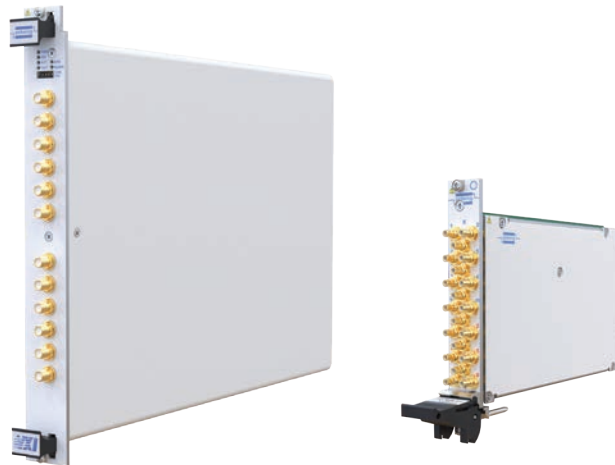
Fig. 5.2 - VXI and PXI Size Differences
