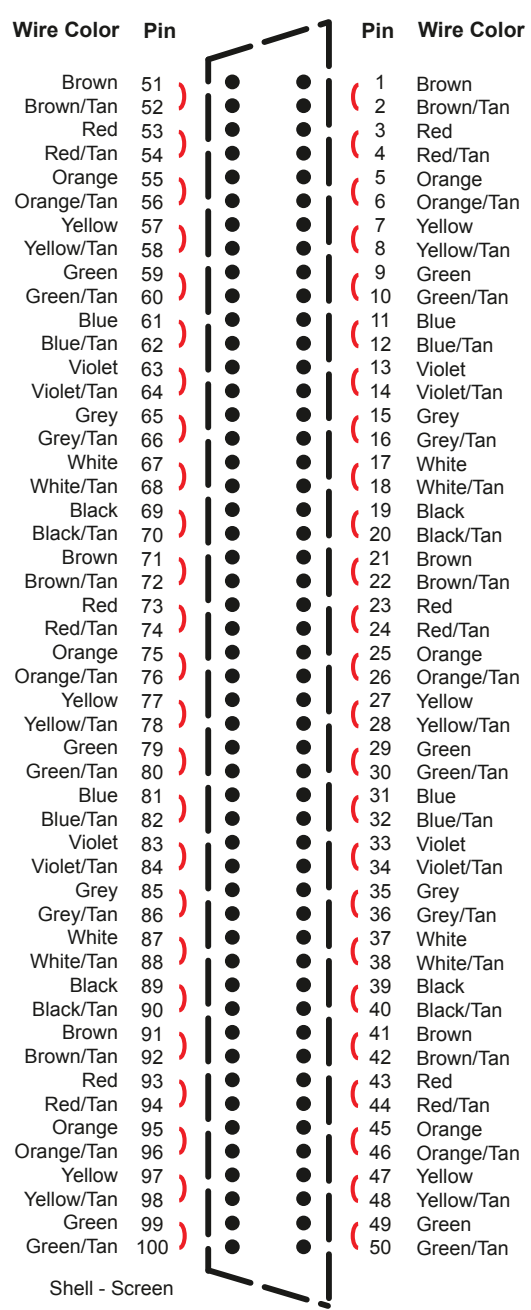
100-Pin 1.27mm Pitch Micro-D Male Connector (Mating Face)
